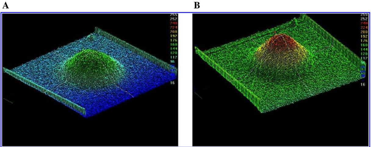
**FIG. 1.** Beam profiles of straight, undamaged, polished optical fibers. (A) The 365- $\mu\text{m}$  fiber. (B) The 272- $\mu\text{m}$  fiber. Both fibers provide near-Gaussian beam profiles.
