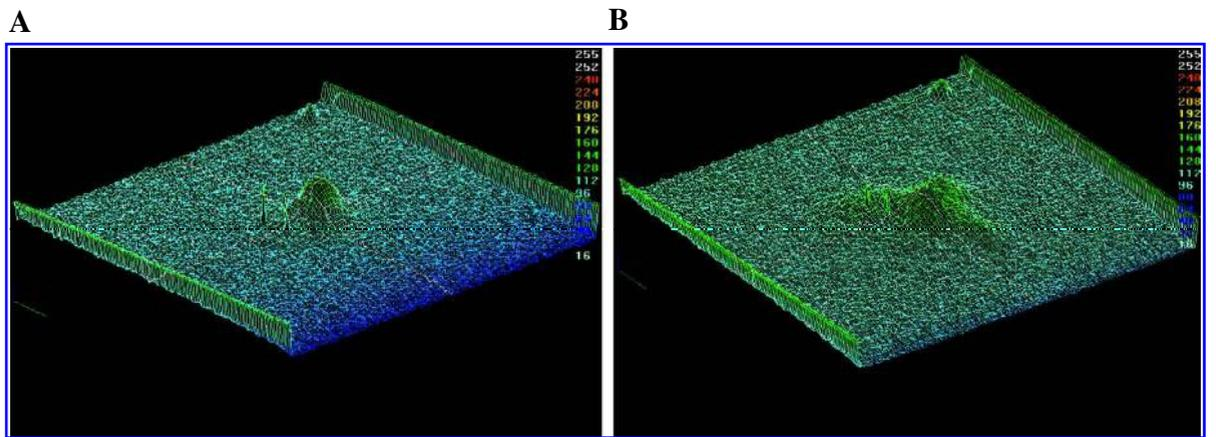
**FIG. 2.** Beam profiles of straight, damaged fibers. (A) The 365- $\mu\text{m}$  fiber. (B) The 272- $\mu\text{m}$  fiber. Both fibers exhibit irregular beam profiles, hot spots, and unpredictable irradiance contours.
