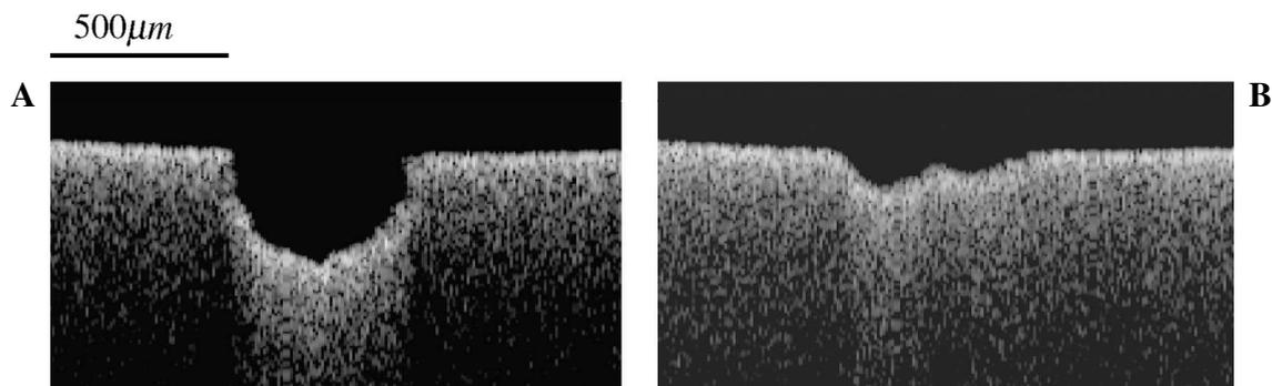
**FIG. 5.** Typical stone crater profiles measured with optical coherence tomography of struvite calculi after single-pulse (600-mJ) irradiation with 272- $\mu\text{m}$  optical fiber. (A) Undamaged fiber produces crater profile similar to near-Gaussian beam profile. (B) Damaged fiber produces an irregular crater with grossly less ablation than is obtained with undamaged fiber.
