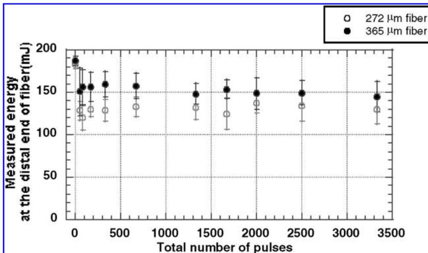
**FIG. 3.** Measured optical output during ablation. There is a rapid decline in measured energy forward of the optical fiber tip within 50 pulses, then relatively steady output of approximately 60% to 70% of stated pulse energy.
